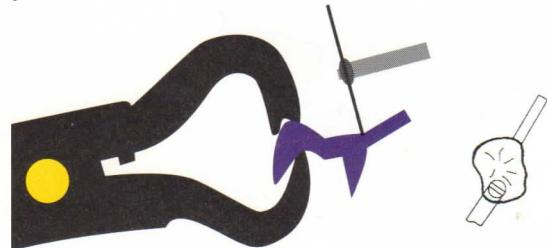
The ideal tool for holding bridges or crowns while separating sprues with a disc.
